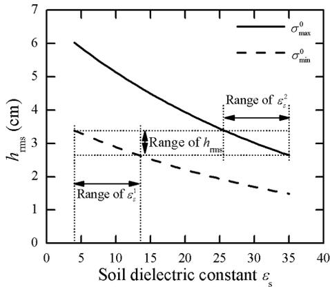
Fig. 1. Ranges of the rms height  $h_{\text{rms}}$  and the soil dielectric constants  $\epsilon_s$  from two SAR measurements.  $\sigma_{\text{max}}^0$  and  $\sigma_{\text{min}}^0$  represent the maximum and minimum backscatter values, respectively.
