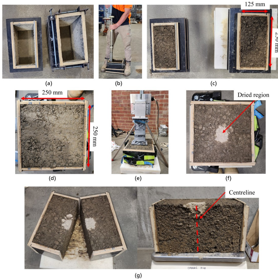
Fig. 2. Experimental stages: (a) two empty wooden moulds; (b) compaction of UGMs; (c) compacted UGMs in two wooden moulds; (d) combined UGM sample; (e) microwave drying of compacted UGM sample; (f) UGM sample after microwave drying; and (g) split UGM sample for data collection
