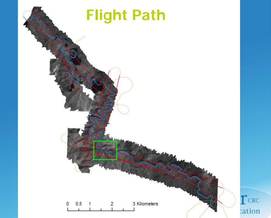
Tri-Spectral Line Scanner  $\approx$  1.0m pixels  $\approx$  1250m swath width Raster files
