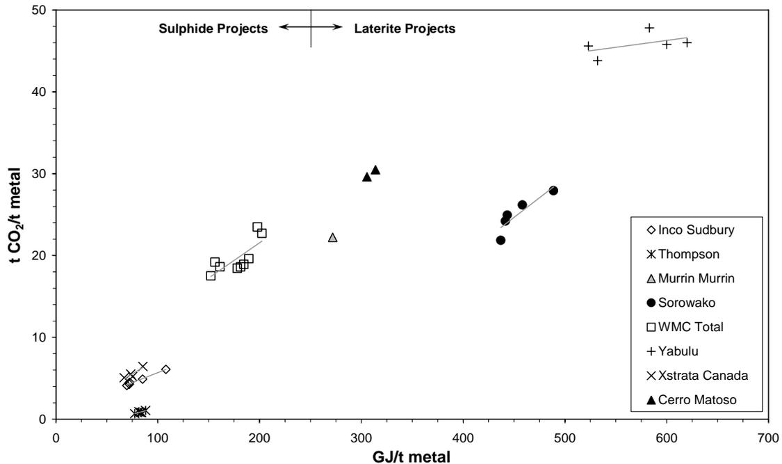
Figure 3 – Carbon dioxide versus energy costs per t metal (Ni±Cu±Co) production (approximate linear trend lines include for some series)
