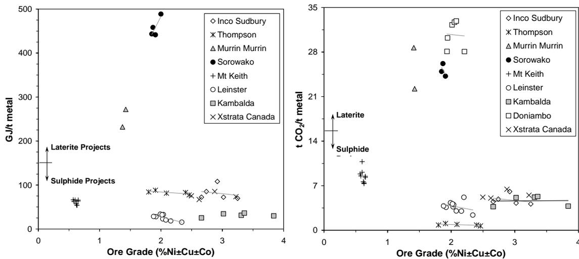
Figure 2 – Unit energy and carbon dioxide costs with respect to ore grade (%Ni±Cu±Co) (approximate linear trend lines include for some series)
