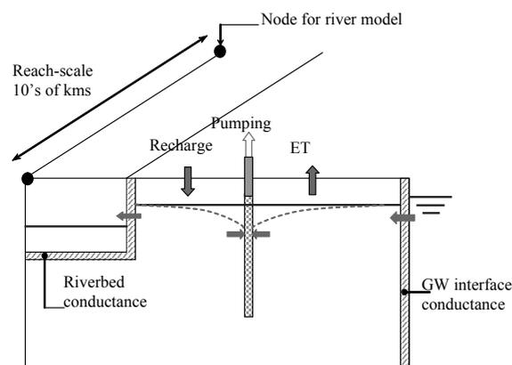
**Fig. 1** Groundwater-surface water interactions for a gaining river system to be modelled in the Groundwater-Surface Water Link Model.
