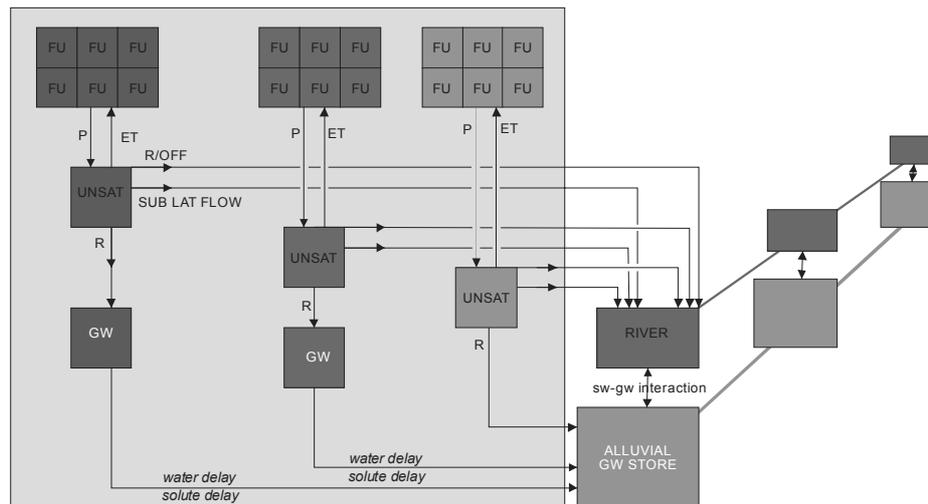
**Fig. 3** WaterCAST structure, showing lumped water balance results for each band, contributing to the river and the alluvial groundwater store. It also shows the connection with downstream river links and downstream groundwater links.
