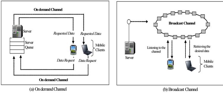
**Fig. 1.** The architecture of on-demand channel and broadcast channel
