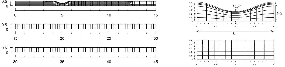
Figure 1: Macro spectral element computational mesh on meridional semi-plane. The full computational domain was extended to  $x = 50D$  with a similar mesh structure to that shown at  $x = 45D$ .
