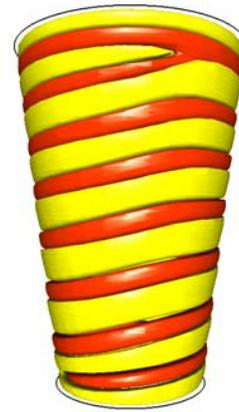
Fig.2. Laminar spirals in the system of conical cylinders.  $Ri=200$ ,  $\alpha=16$  degrees,  $\eta=0.84$  at the top of the system,  $\Gamma=H/d=12.50$ . ( $H$  is the height of the fluid column,  $d$  the gap and  $\alpha$  the total (apex) opening angle of the conical cylinders). Isosurfaces show +/- radial velocity
