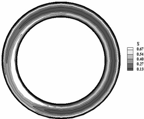
Fig.5. Representation of vorticity contour lines at an axial cross section in finite cylinders geometry. The section is taken at the location of the vortex dislocation separating the top Ekman vortex from the spiral vortices taking birth below.  $Ri=300$ ,  $Ro=0$ ,  $\eta=0.75$ ,  $\Gamma=12.98$ .
