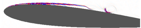
Figure 6. Optimal two-dimensional initial perturbation for \tau = 0.25T visualized with contours of spanwise vorticity. 100 contour levels are used between \omega_z = \pm 10\% of maximum.
