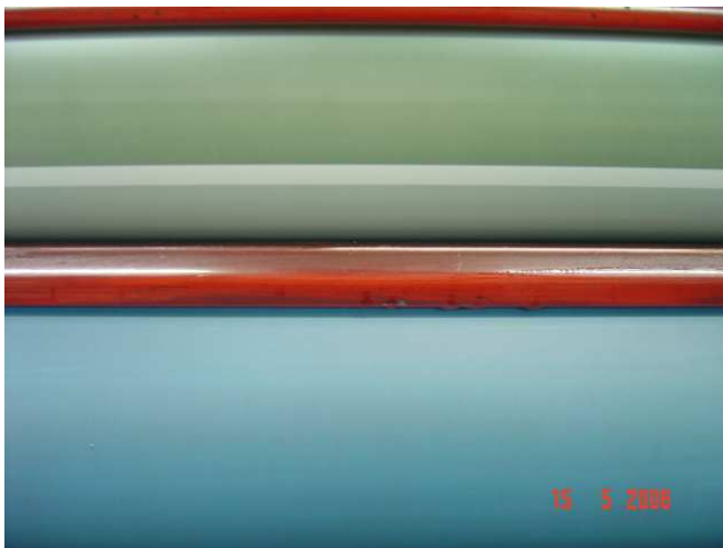
Figure 5. 31. Diazo plate was worn out after 7000 copies were printed
