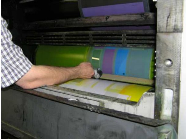
Figure 3. 15. Application of Tape to the Blanket
