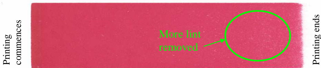
Figure 3. 3 More lint removed in latter part of IGT Printed samples, despite constant printing speed [8].
