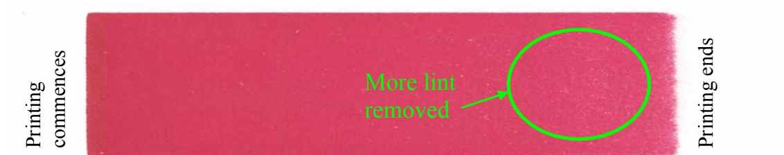
Figure 3.1 – More lint removed in latter part of IGT Printed samples, despite constant printing speed
