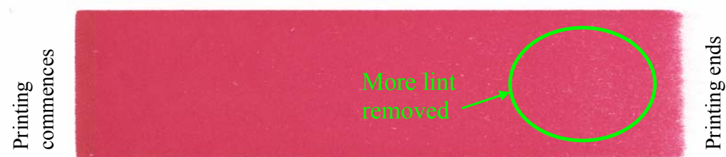
Figure 3.1 – More lint removed in latter part of IGT Printed samples, despite constant printing speed
