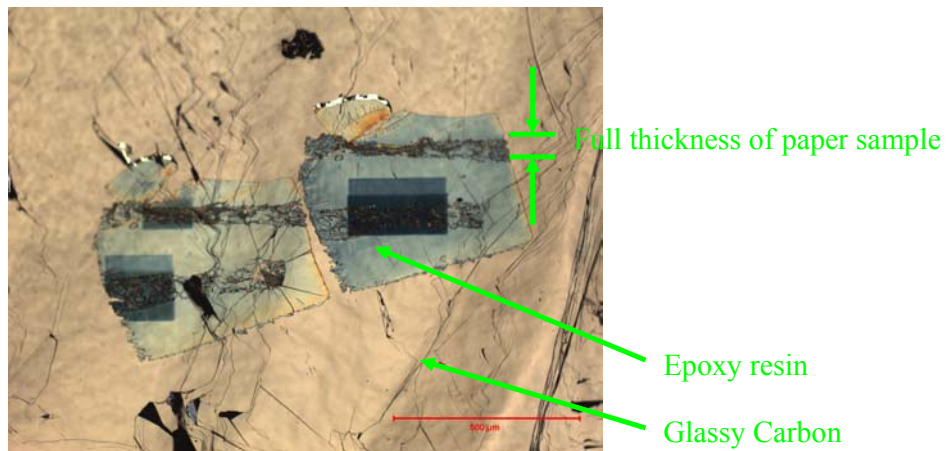
Figure 3.28 – 100X Four cross-sectioned samples of newsprint for SE Microprobe
