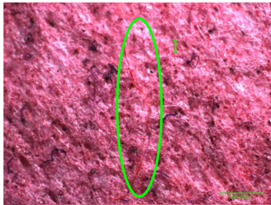
Figure 3.9 – 50 X View of lint particles, including a cotton fibre. The scale marker represents 500 μm.
