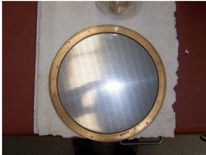
**Figure 3. 7: Slotted screen (0.2mm)**
