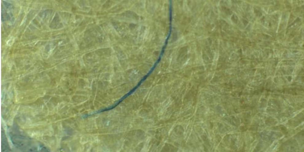
**Figure 3. 13: Dyed fibre observed under the Olympus BX 60**
