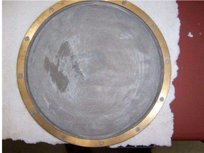
**Figure 3. 8: Screen (200 mesh) used for removal of fines**
