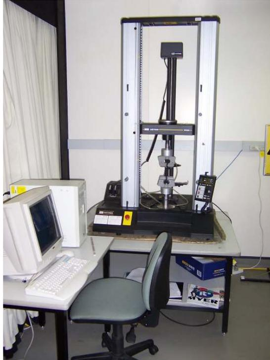
**Figure 3. 20: Instron Tensile tester 5566**
