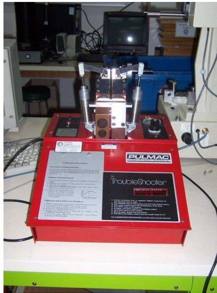
**Figure 3. 22: Zero Span Tensile Tester**
