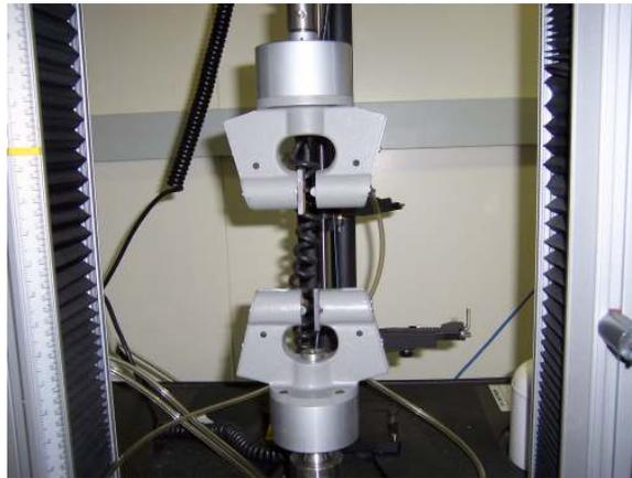
**Figure 3. 21: Jaws of the Instron Tensile tester**
