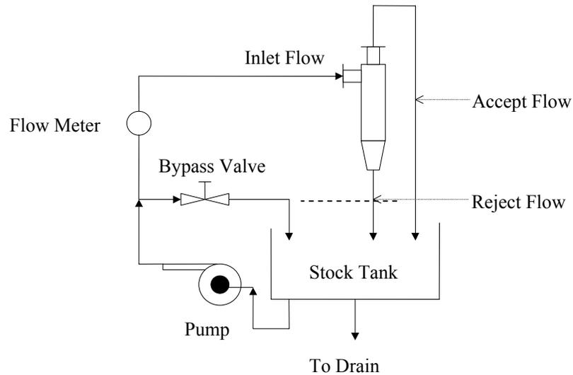
**Figure 5-3 Hydrocyclone unit used in the fractionation experiment.**
