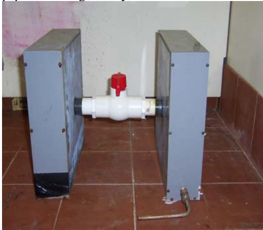
Figure 1: Acid Exposure Chamber Assembly
