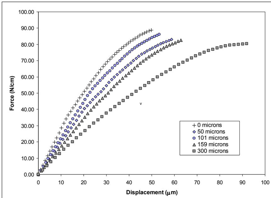
Fig 1. Average load-displacement curves determined for tests on sample B refined to 1000 PFI revolutions. The legend indicates the short span at which the test was conducted. The zero microns data is for the zero-span test.
