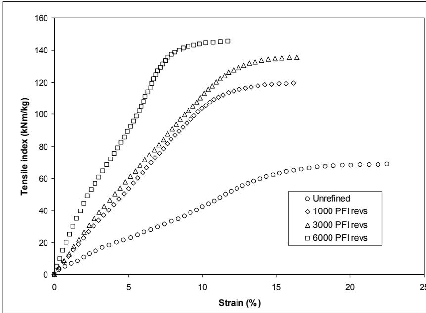
Fig. 5. Cross-section stress-strain curves of paper made from unrefined and refined previously dried, bleached softwood kraft pulp (C)
