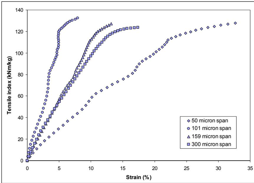
Fig. 2 Stress-strain curves determined for sheets made from bleached pulp B refined to 1000 PFI mill revs.
