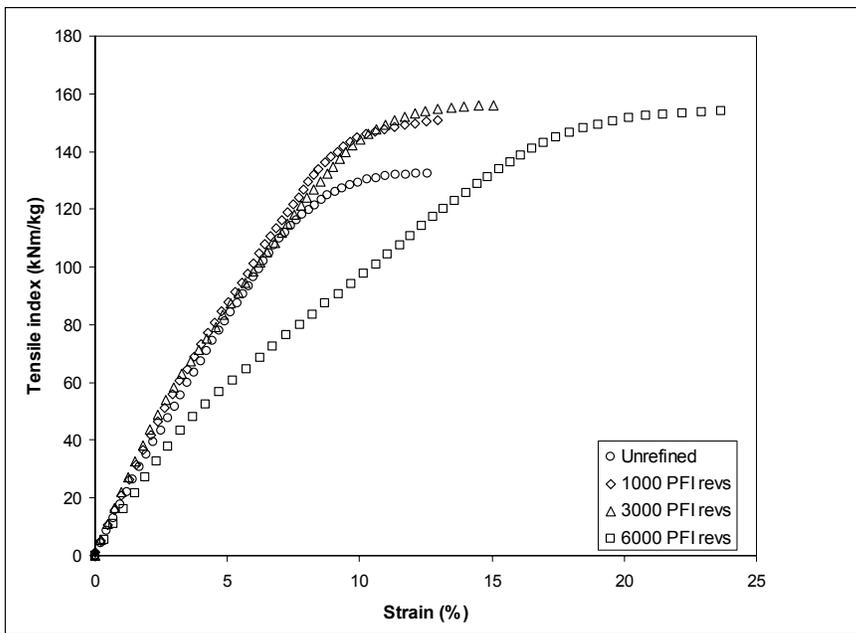
Fig. 3. Cross-section stress-strain curves of paper made from unrefined and refined unbleached softwood kraft pulp (A)
