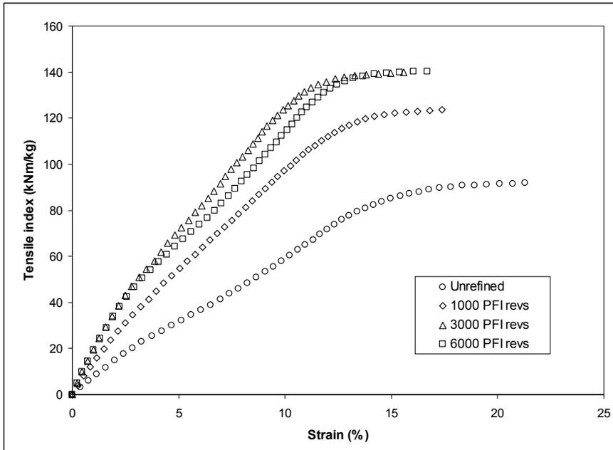
Fig. 4. Cross-section stress-strain curves of paper made from unrefined and refined bleached softwood kraft pulp (B)
