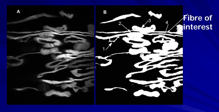
Cross-section image before (A) and after (B) thresholding and binarisation. Fibre 2 and 3 in (B) make two full contacts, fibre 1 makes a partial contact, and fibre 4 is not in contact with the fibre of interest.
