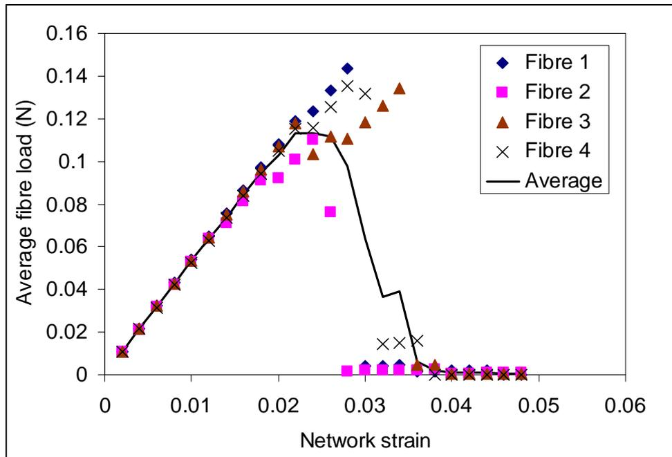
Figure 2 Simulation of the debonding of four fibres of the LO-P3 sample.
