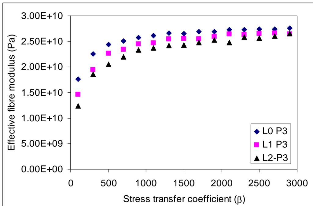
Figure 1. Effective fibre modulus as a function of stress-transfer coefficient with assumed fibre elastic modulus of  $3.0E+10$  Pa. Length weighted fibre lengths were 3.14, 2.53 and 2.10mm for LO, L1 and L2, respectively.
