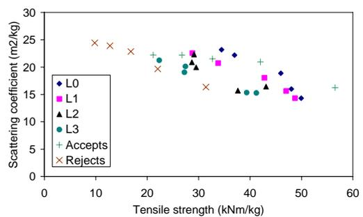
**Figure 2 Scattering coefficient versus tensile strength for the APPI data**
