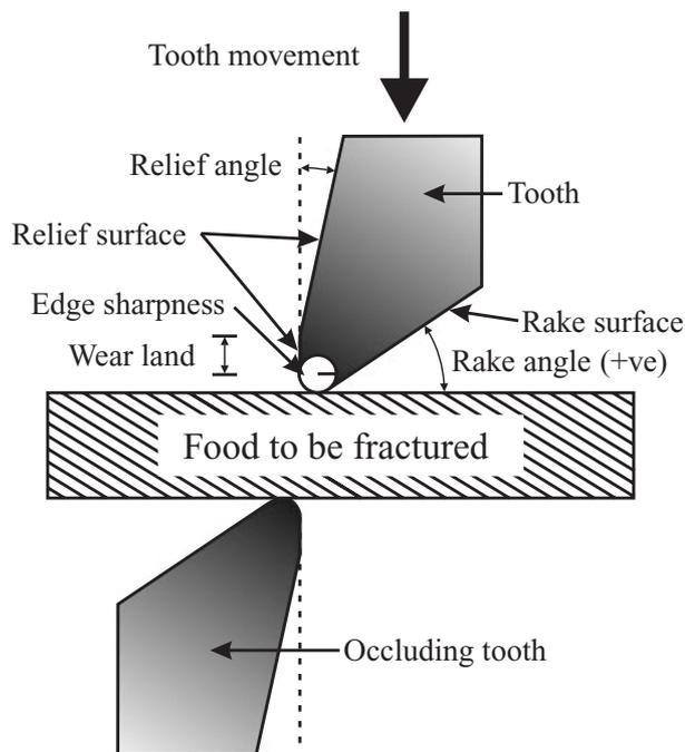
**Figure 1.** Rake angle, relief angle, wear land and edge sharpness of a crest viewed end-on. The circle radius indicating edge sharpness is enlarged for clarity, and is much smaller in actuality.
