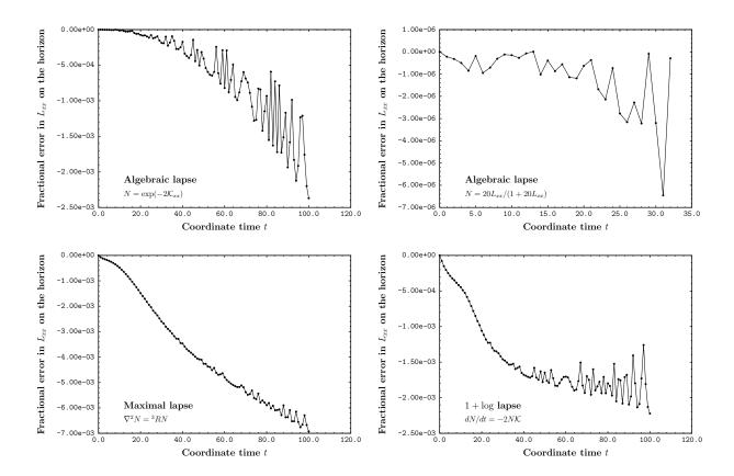
**Figure 8:** In the absence of gravitational radiation the area of the horizon should remain constant. It follows that the  $L_{xx}$  should be constant on the horizon. Here we plot the fractional variation of  $L_{xx}$  on the horizon. The irregular behaviour of the plots for later times is due, in part, to the difficulty in accurately locating the horizon.
