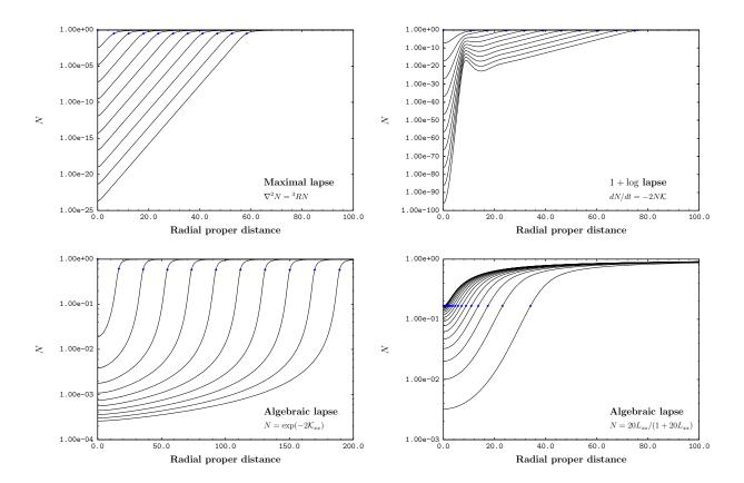
Figure 6: As per figure (5) but this time we display the lapse profiles. Note how quickly the lapse collapse at the throat in the  $1 + \log$  slicing. This would likely cause serious underflow problems for  $t \gtrsim 300$ . Notice also the uniform spacing of the curves along the logarithmic axis for the maximal lapse. This show that the lapse collapses exponentially at the throat (a well known result for maximal slicing).
