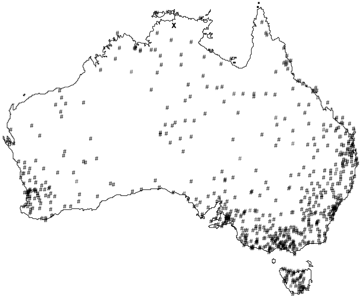
Figure 5.7 Locations of stations used in evapotranspiration analyses by Morton’s Method (Chiew et al. 2002). The location of the site is indicated by ‘X’ in the map
