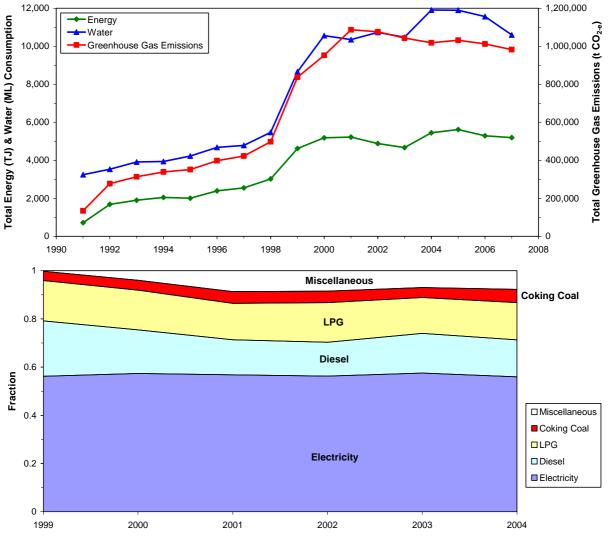
Figure 5: Annual energy consumption and greenhouse gas emissions for Olympic Dam (top) and energy source by fraction (1999-2004; bottom)
