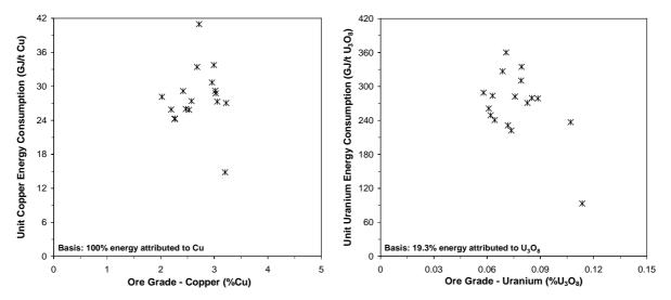
Figure 7: Unit energy consumption versus ore grades - copper (left) and uranium (right)
