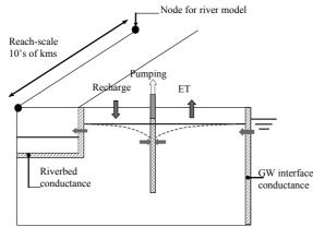
Fig. 1 Groundwater-surface water interactions for a gaining river system to be modelled in the Groundwater-Surface Water Link Model.
