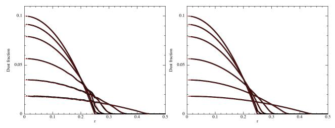
**Figure 4.** Dust fraction as a function of spherical radius in the 3D dust diffusion test at t = 0.0, 0.1, 0.3, 1, 3 and 10 (top to bottom) from simulations using  $50 \times 58 \times 60$  particles. The numerical solution, projecting all particles in r, is given by the black dots and may be compared to the analytic solution given by the red lines. The left panel shows the solution with two first derivatives, while the right panel uses the direct second derivative.
