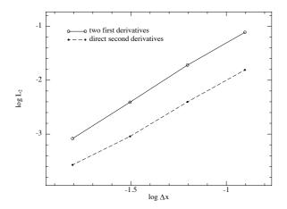
Figure 6. Convergence in the dust diffusion problem, showing  $L_2$  error for the solution within r < 0.2 as a function of the particle spacing. While both methods show second order convergence, the direct second-derivatives solution is more accurate because of oscillations in the two first derivatives approach propagating from the 'kink' in the initial  $\epsilon$  profile seen in Figure 4.
